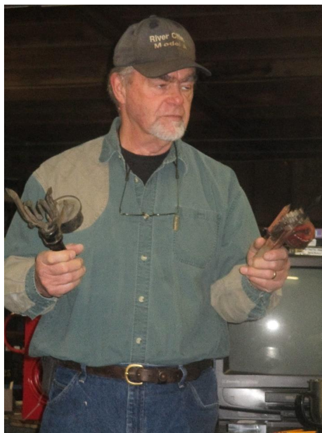
Bobby displayed two early testers to check the condition of batteries under load.
