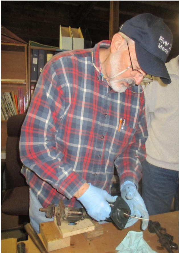
Joe is intent on cleaning all lubrication passages. Note the wire he is using.
