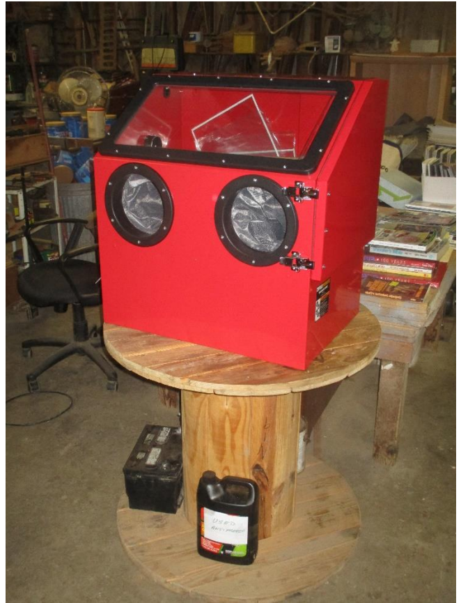
The parts disassembled and cleaned will be sand blasted in this unit and then painted during the April session.
