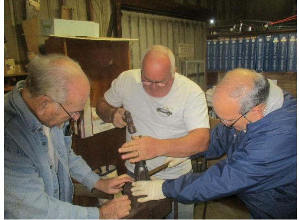
Larry is driving out a pump shaft as Joe and Al hold the casting steady.
