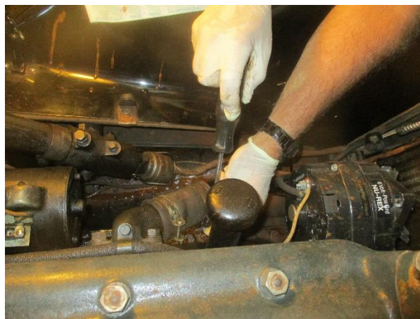
Removing the engine's water return hose.
