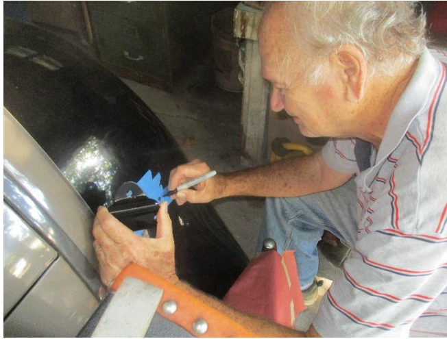
Joe Spooner locating the hole for the new stop light. Sharon said measure twenty times Joe and drill once!
