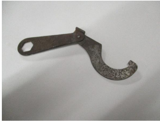
Jim Langley passed around an original water pump wrench. Note that it folds.
