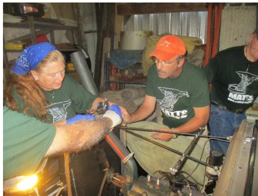
Getting down to work. Many hands help remove the radiator from Sharon's 31 Coupe.
