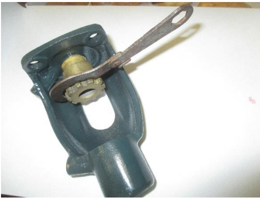
Jim Langley passed around an original water pump wrench. Note that it folds.
