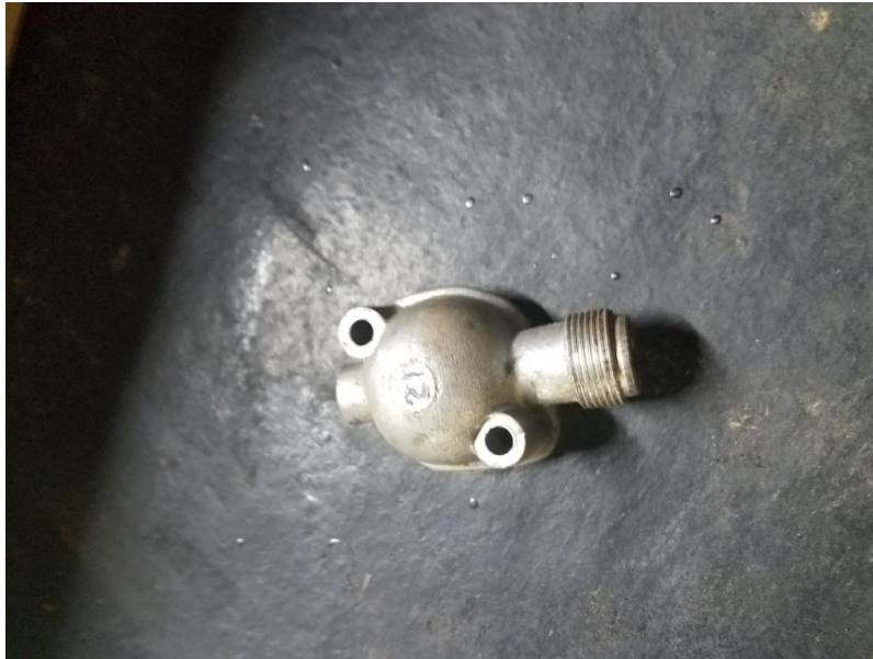
Showing the back side of one of the speedometer gear caps...
