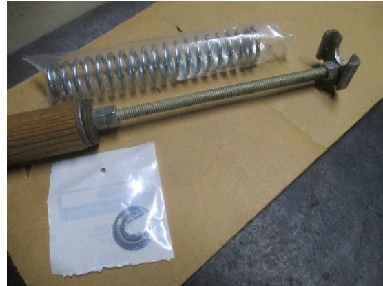
Gear Shift Lever Spring Remover tool made by Bobby Penny. Also see a replacement spring.
