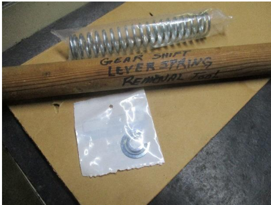
Gear Shift Lever Spring Remover tool made by Bobby Penny. Also see a replacement spring.
