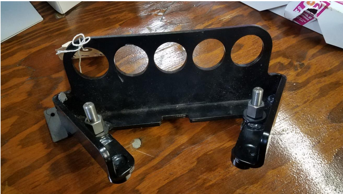
"Al shows one of the tools used to remove an engine head. This tool can also be used to remove or install an engine" ...
