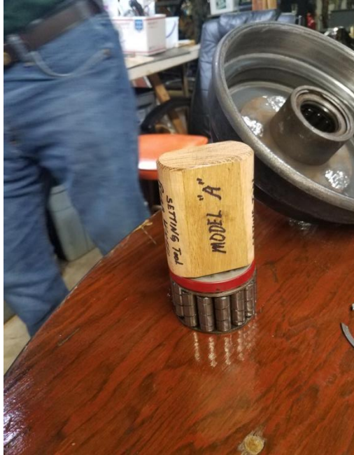
"A homemade tool used to insert bearings into the drum" ...
