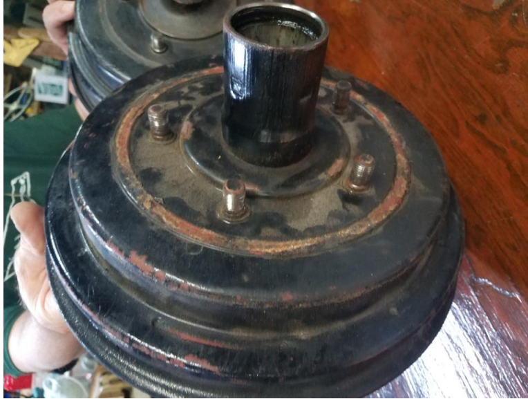
“Studs correctly placed in drum” ...
