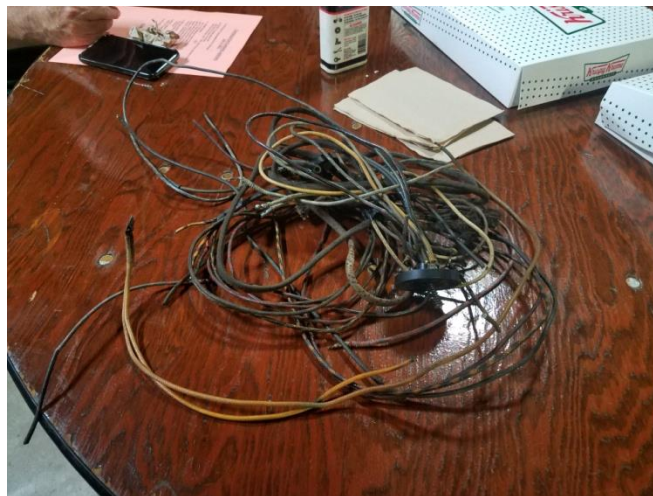
"This is how the wire harness looked on one of Bobby's newest Model A's. He will replace it with a new wire harness" ...
