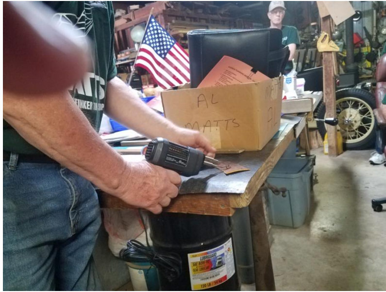
"Using a piece of leather to solder wires" ...
