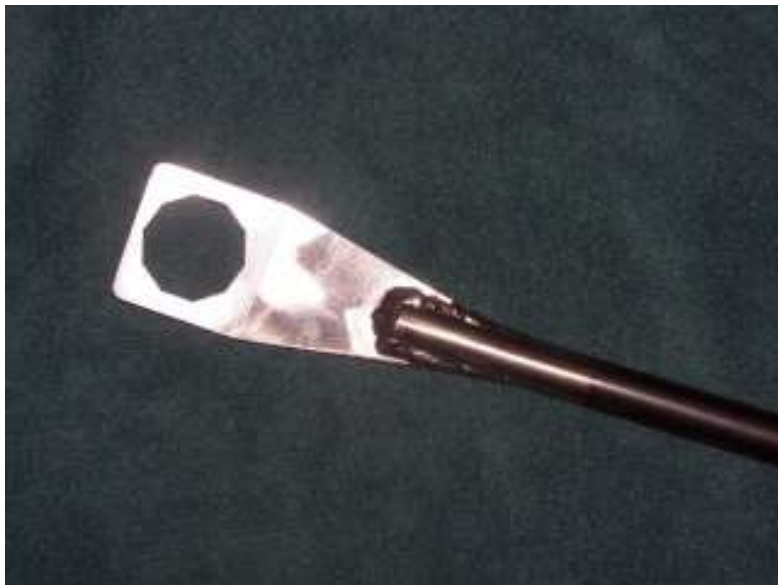
"Having problems removing the outer ring of your gas gauge? Al has made this tool with an extended handle to make removing it easier"...
