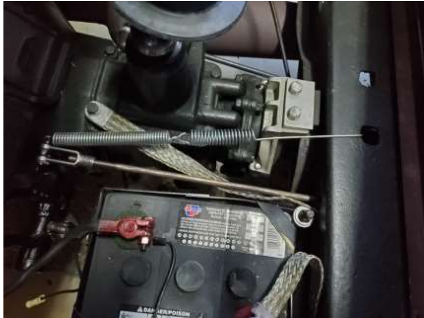
“Al Lugo showed pictures of the brake return spring he places in his Model As” ...
