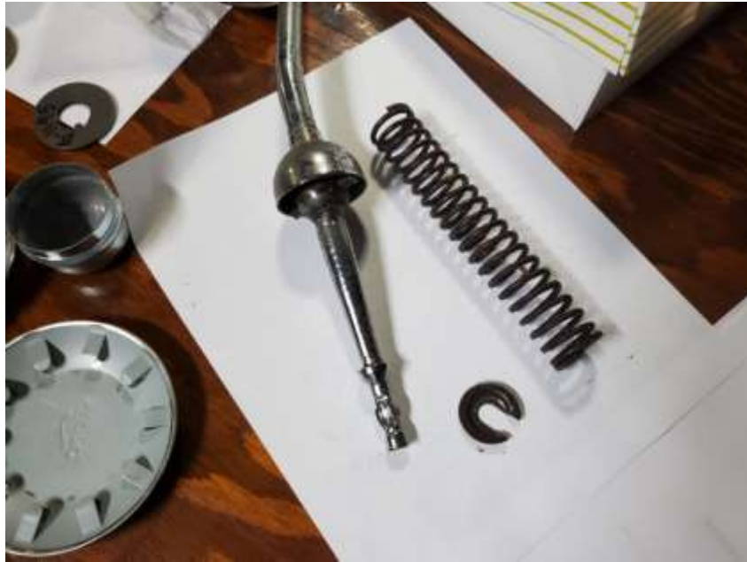
“AFTER AL HAD A PROBLEM PLACING THE RETAINING CLIP, BOBBY SHOWED THE COMPONENTS AND THE PROPER PLACEMENT” ... “Photo by Al Lugo”
