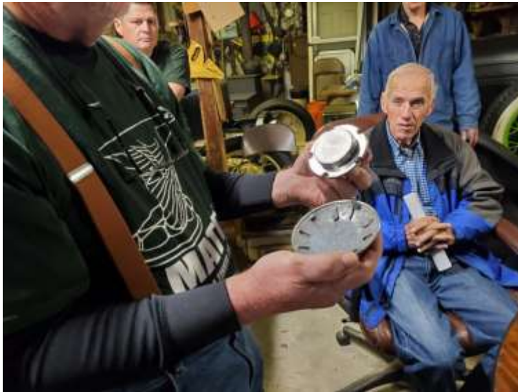
"BOBBY SHOWS A TOOL AL PURCHASED TO MAKE INSTALLATION OF 30/31 HUB CAPS EASIER AND SOME OF THE PROBLEMS WITH SOME OF THE HUB CAPS HE FOUND" ... "PHOTO BY AL LUGO"
