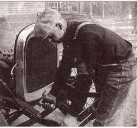
Always grip the crank with the thumb wrapped below with the fingers. NEVER push the crank down the right side of the rotation!
