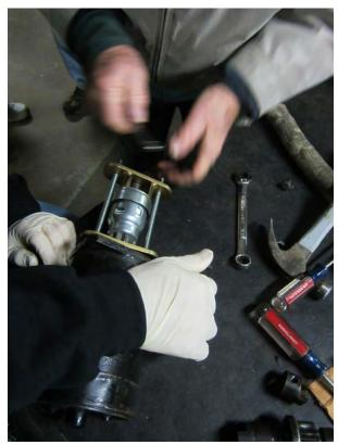
A Modern Starter Drive is being installed. This drive has a self contained spring ensuring screws and washers can't fall into the flywheel housing.
