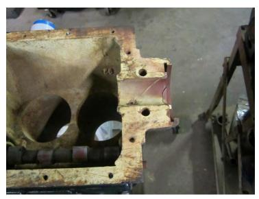
A stripped down Model A engine block is displayed at MATTS. Here clearly shown is the upper block portion of the Rear Main Bearing with babbitt.
