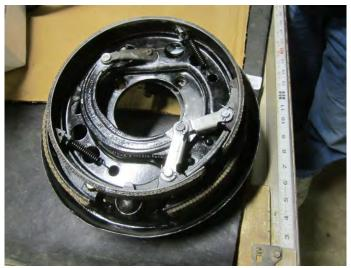
A rebuilt Rear Brake Assembly with service And parking brake linings, is ready for installation on a waiting Model A.
