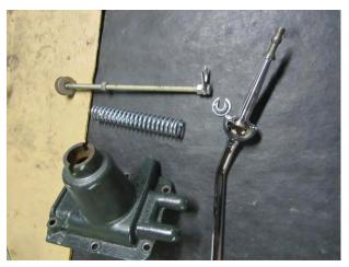
Here is a dissembled Transmission Tower. A powerful spring must be removed and reinstalled during the rebuilding process. A special tool is essential to prevent possible injury. Note only part of a tool is shown in the above photo.
