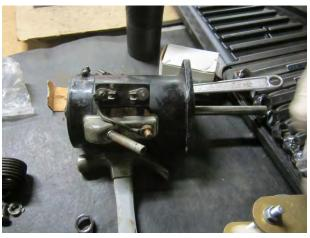
Here the original Bendix Starter Drive has been removed from a starter.
