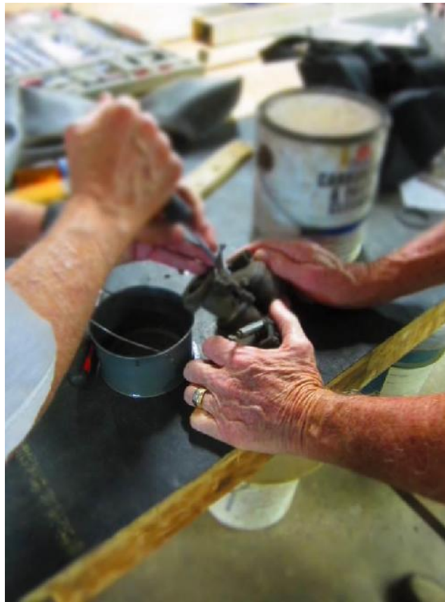
Members disassembling a carburetor prior to placing it's parts in the nearby basket for immersion in carburetor cleaner.
