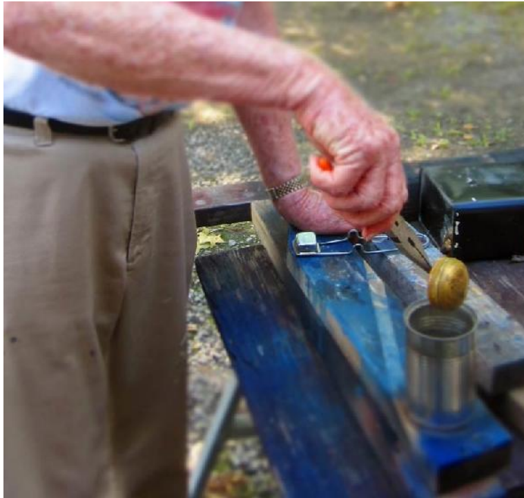
Members disassembling a carburetor prior to placing it's parts in the nearby basket for immersion in carburetor cleaner.
