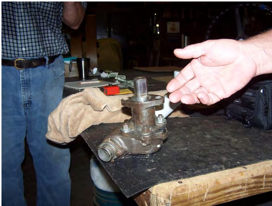
Bobby shows the project for the day: How to restore the Model A Steering box.
