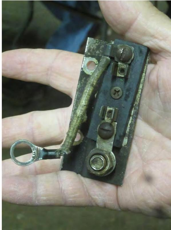
**The after market fuse block had loosened which resulted in loss of electrical power to the engine. Larry and Bob Smith found the problem and corrected it to get the pickup back on the road.**
