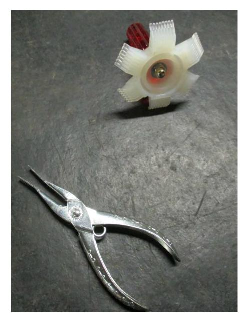
Bent radiator fins can be quickly straightened with these tools Al got from Harbor Freight.
