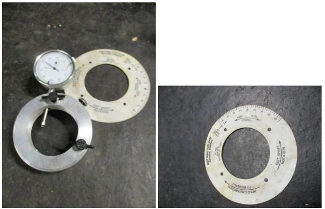
Mechanical or adjustment problems can be diagnosed and fixed with the club distributor measuring fixture.
