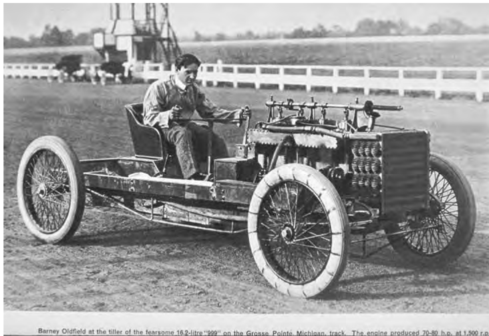
Barney Oldfield at the tiller of the fearsome 16.2-litre "999" on the Grrosse Pointe, Michigan, track. The engine produced 70-80 h.p. at 1,500 r.p.m.
