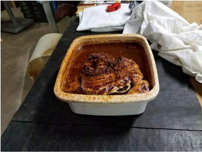
This is how the container with Paul Singer's Rusty Carburetor looked after some time in Vinegar and water...
