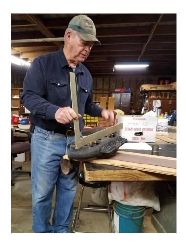
Shown here is Bobby checking the level and flatness of an exhaust manifold.
