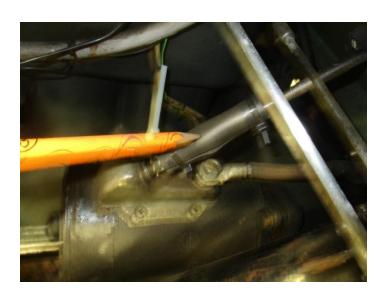
Insulation of the Starter Rod with a length of hose to prevent accidental contact with it when connecting a battery charger to the "Hot" Starter Motor contact. (Info from Tiny Tips of the <u>Restorer Magazine</u>
