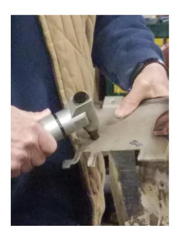
A pneumatic nibbler is shown here cutting thin gage sheet metal. The nibbler was the fastest cutting tool.
