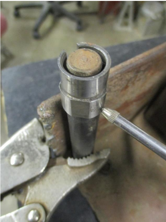
A simple measuring jig was made to check the rise of each cam lobe.
